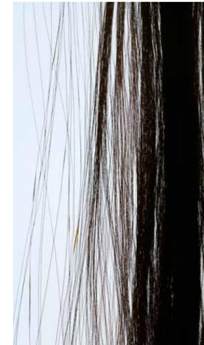
Lightweight carbon fibers from lignin from pulp mills
