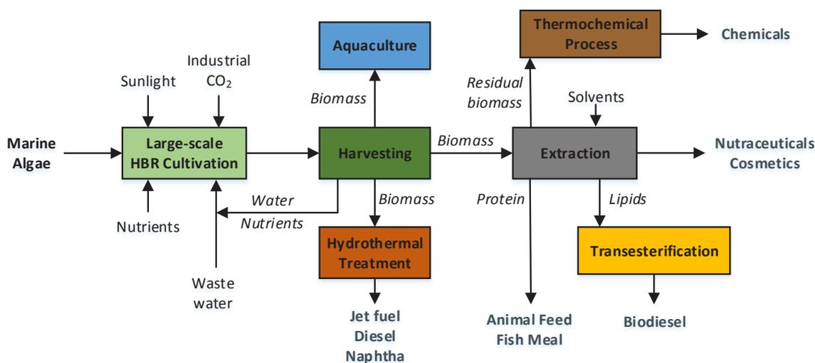
**Fig. 1.** Block diagram of an envisioned potentially more sustainable and cost-effective process for manufacturing a portfolio of algal biofuels and bioproducts via a low-cost modular bioreactor (HBR), wastewater use, nutrient reclaim, and recycling loops in an industrial setting.
