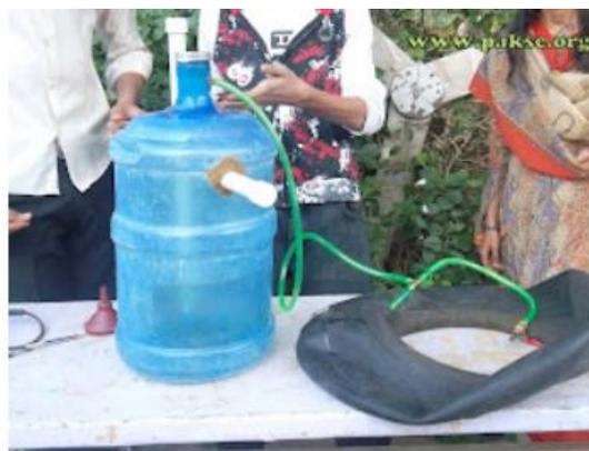
A biodigester setup where biogas inflates a rubber tire
