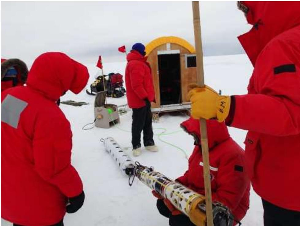
*Caption: The SCINI ROV (in foreground) is being tested by a researcher prior to deployment, while the acoustic towed package is the white cylinder laying on the snow behind it. The Conestoga wagon “dry lab” is in the background. Photo credit: Stacy Kim.*
