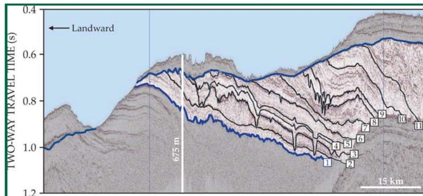
**FIGURE 2. A SEISMIC PROFILE** tells the history of glacial ice on the Sabrina Coast continental shelf, now underwater. The region between the two blue lines represents a period when the ice was responding dynamically to fluctuations in climate; each of the bold lines marked 1–11 is an erosion surface created by glacial advance and retreat. (Adapted from ref. 1.)
